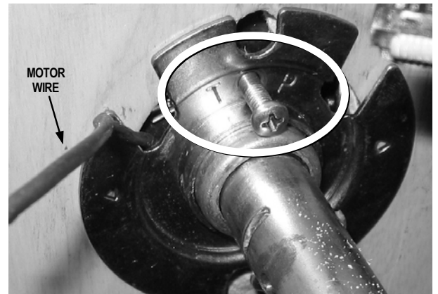
FIG. 12: INSIDE ROSE PLATE INSTALLATION
