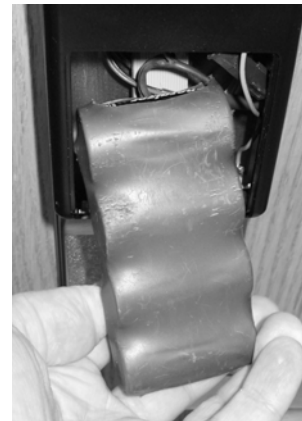
FIG. 18: INSERT BATTERY PACK INTO HOUSING
